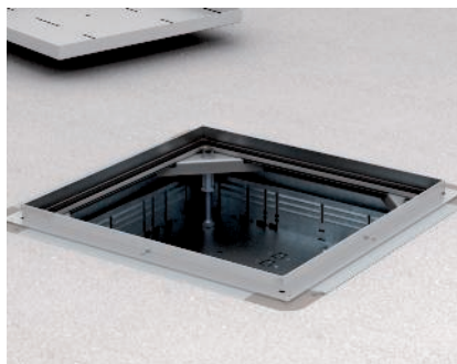
Mounting of lid heavy-duty support Insert the four heavy-duty lid supports in the corners of the underfloor box and adjust them to the required height. Lock the support screw with a locknut.
