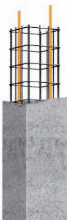
Example: use of reinforced concrete supports/ down-conductor system
