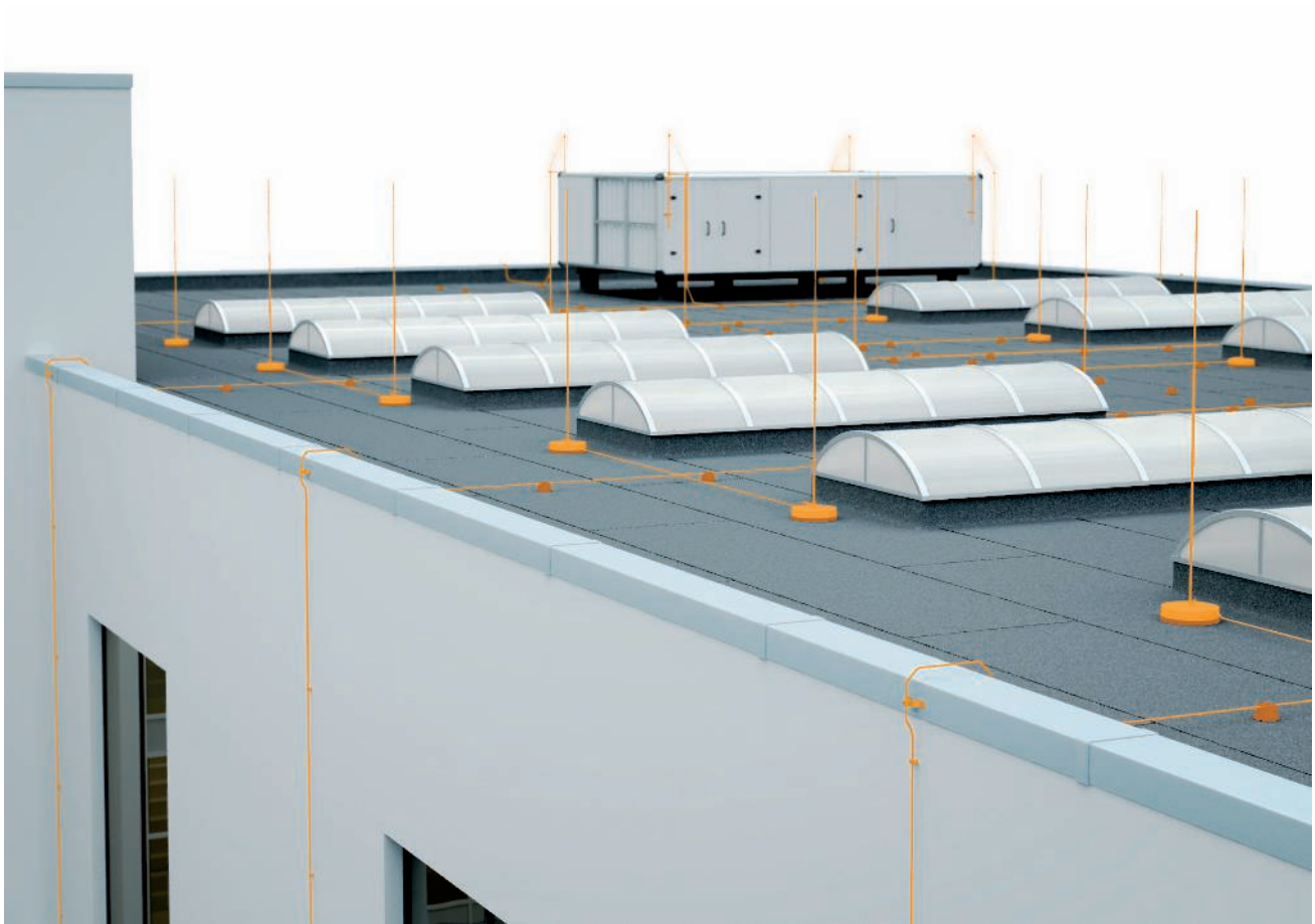
Natural components (here: metal of roof parapet) for air-termination systems, IEC 62305-3
