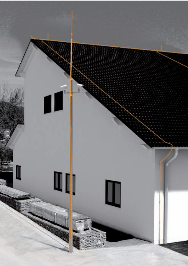
CCTV cameras with isCon® conductor
