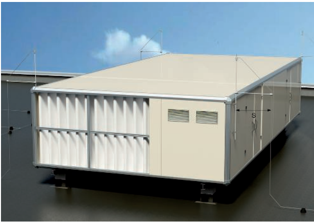
Insulated air-termination system with separation distance (s)
