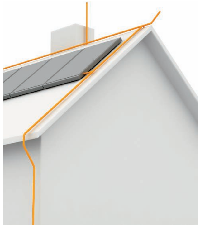
Direct connection of the PV mounting frames to the lightning protection system
