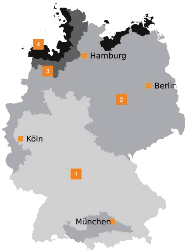
Wind zones according to DIN EN 1991-1-4/NA
