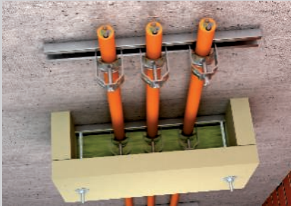
Effective support measure with ZSE90 strain relief.
