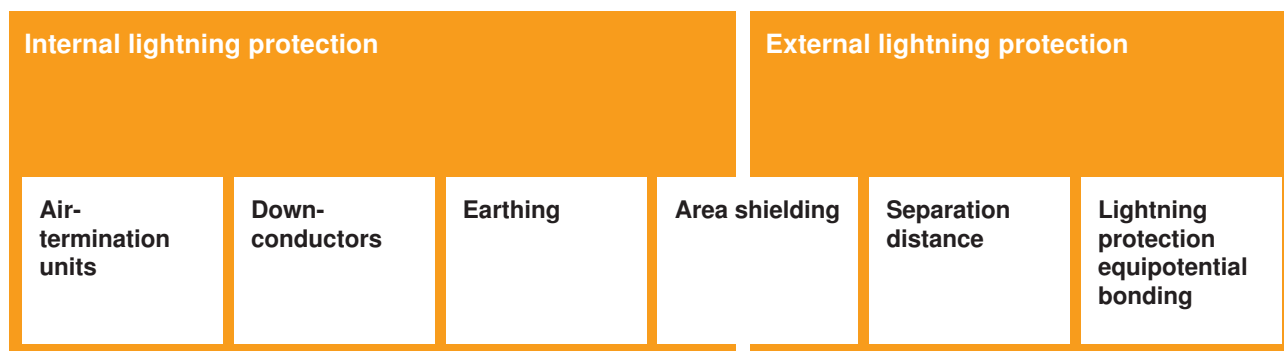
External and internal lightning protection systems
